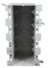
EZ68QO EZ BOX is a 4-Gang, 68 cu. in., renovation application (old work) electrical switch or outlet box for residential or light commercial renovation projects when a 4-gang box is needed. EZ mount flanges, winged swing tabs and built in wire clamps make installation easy and cost effective.
